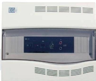
1301.1 Audio processor is the main module of the installation and has been designed for in-wall mounting. It has 2 amplifiers (20W / 10W) and a 15 V $\overline{\text{=}}$  line output to connect the autoamplified control units. It also includes door-opener, FM tuner, and RCA connectors to connect the external audio source.
