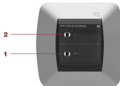
**40140** Auxiliary module has one stereo audio input (**1**) through a 3.5 mm jack connector. It allows the connection of an external audio source using the **EGi** wire of ref. **0501** or **0503**. It also has one stereo headphones output (**2**).
