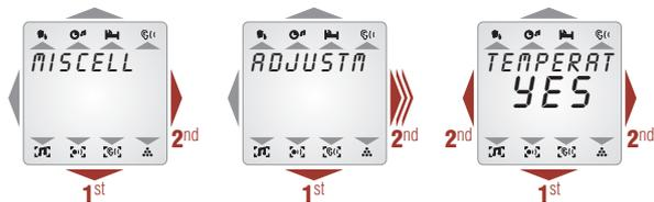
Although the probe is calibrated, it might be possible that you have to adjust the probe for optimal performance.
